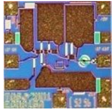
High Speed VCSEL driver chip (25 to 40Gbit/s)
